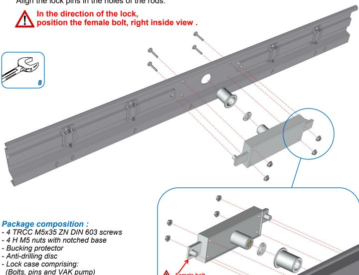
2) Fasten the whole with the screw kit, included in the lock package.
