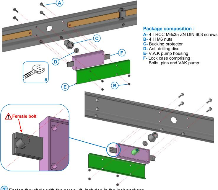
2 Fasten the whole with the screw kit, included in the lock package.
