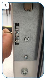
Once open, return to the : Box operation test section and set the latches correctly by following the test steps.
