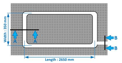
Loop perimeter = **6000 mm** Connecting cable = **9000 mm**
