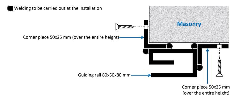
If the reinforced clamps are welded onto the guiding rail : The corner piece of 50x25 mm must be recut, in order to fix it between the clamps.
