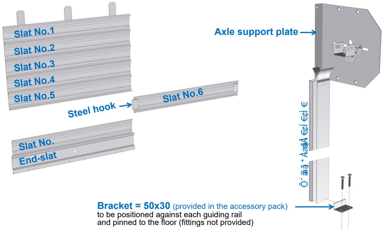
**No. of slats with steel hooks, for axle of Ø220 mm**
