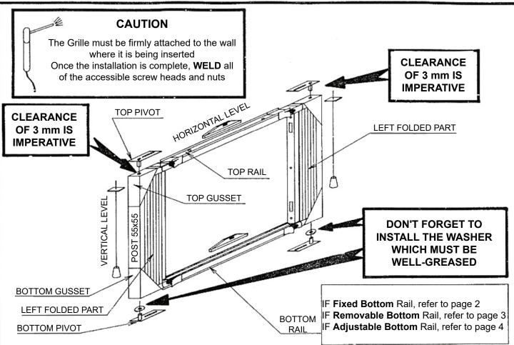
The axle of the top **PIVOT** and the axle of the bottom **PIVOT** must be plumb and correctly aligned:
