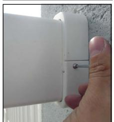
Attach the Rail using the hollow hex screws M5x8, until pressurized. These screws enable the support to be locked in place.
