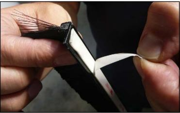
Attach the weather seal section to the column and press it down firmly.
