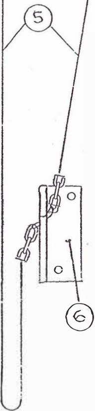
POSITION THE HAND CHAIN TO MAINTAIN THE SHUTTER AT ITS MAXIMUM OPENING POSITION (BACK STOPS COMPRESSED BY 10CM)
