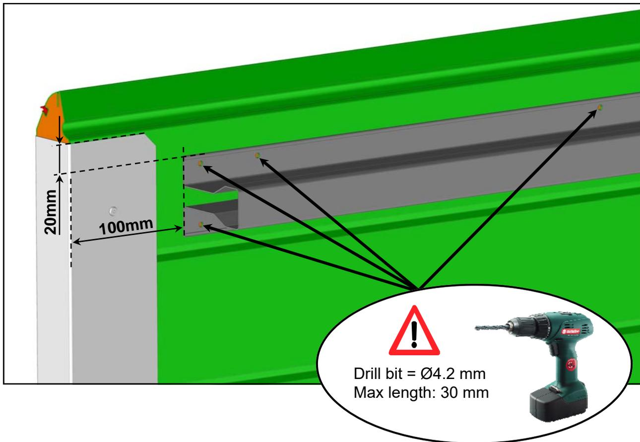
B) Attach the Oméga stiffener with the peel rivets.
