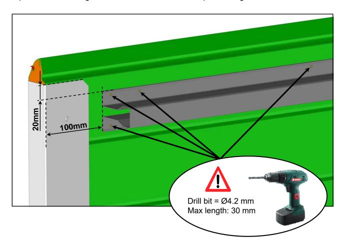
B) Attach the Oméga stiffener with the peel rivets.
