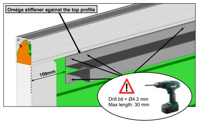
B) Attach the Oméga stiffener with the peel rivets.
