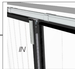
Clearance side Lip seal or brush seal depending on reservation dimensions
