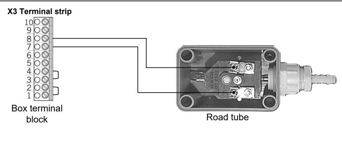
Before connecting the Road tube, ensure that all of the instructions in the connection manual for the PIC 4410, Intellidrive 400 or CS 300/310 boxes have been followed.
