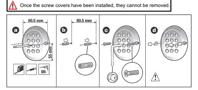
2 - Attach the electric box to the wall in accordance with the diagrams below.
