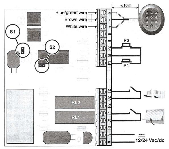
If **S1** is not equipped with a jumper **(a)**, the lights on the keypad will switch on for 10 seconds after having pressed any key.
