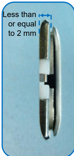
The latches should only come out as far as 2 mm or less
