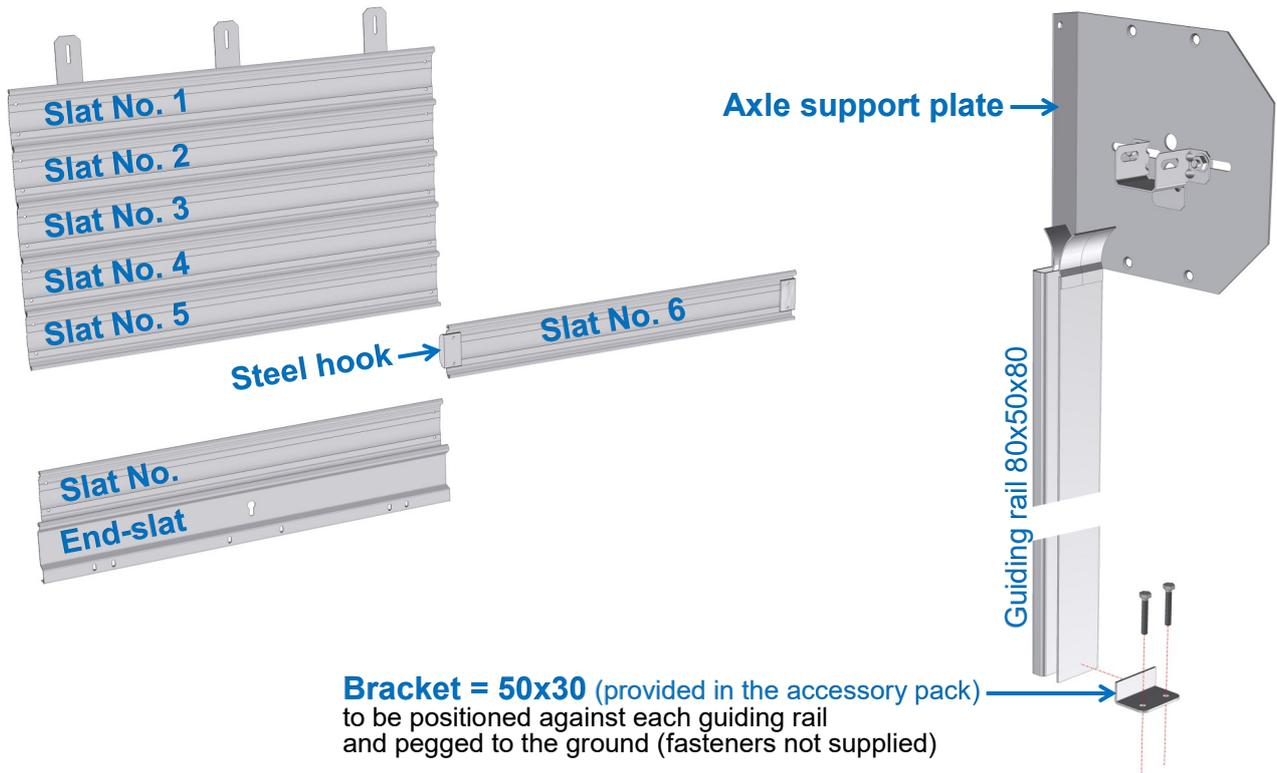
**No. of slats with steel hooks, for axle of Ø168 mm**
