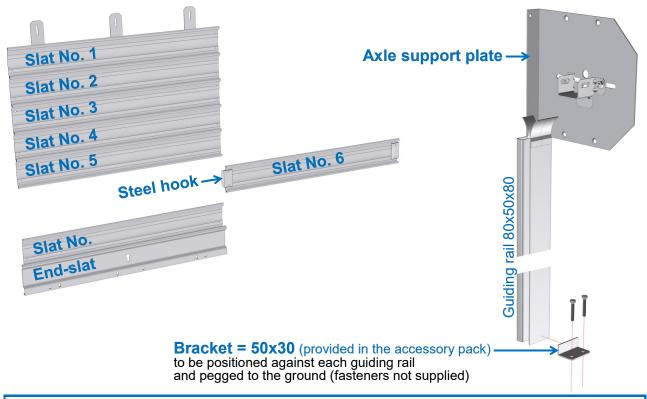
No. of slats with steel hooks, for axle of Ø168 mm 6 - 11 - 16 - 21 - 26 - 31 - 35 - 37 - 41 - 44 - 47 - 51 - 55 - 59 - 64 - 68 - 73 - 77 - 82 - 86 - 91 - 96 - 101
