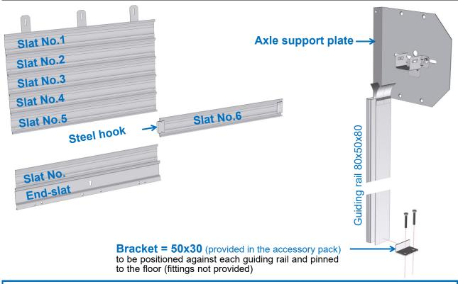
No. of slats with steel hooks, for axle of Ø193 mm 6-11-16-21-26-32-36-38-42-46-49-53-57-60-64-68-73-77-82-87-92-98-102
