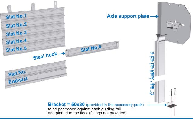
No. of slats with steel hooks, for axle of **Ø273** mm 6-11-16-21-26-28-32-37-39-44-49-54-59-64-69-74-79-84-90-94-99
