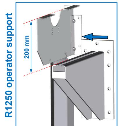
Firmly attach the support to the wall with the steel pins and 6 TH M14 screws (pins and screws not provided).
