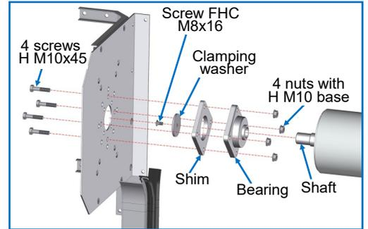
**5- Installing the operator :** Stick it on the keyed shaft.
