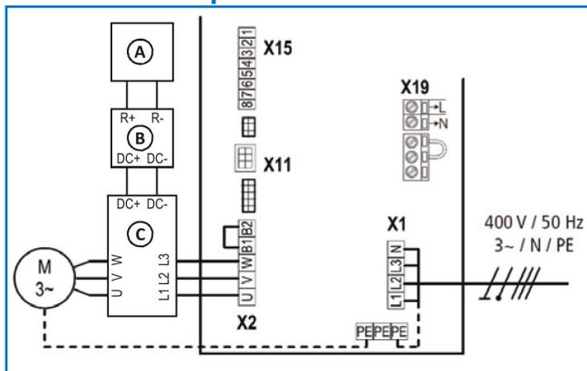
(A) Braking resistor.
