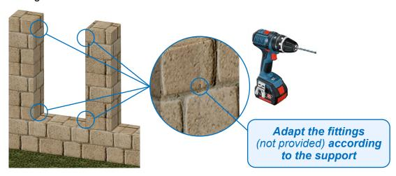
Reposition the fence element, according to the dimensions and attach it :
