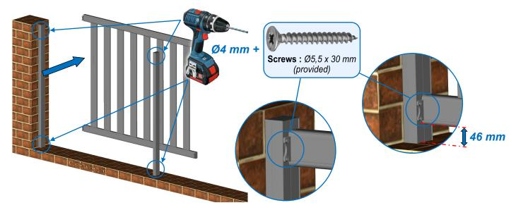
Support the fence element and repeat the process from the section: Position the fence element and draw the fitting points, to fit the following fence elements.
