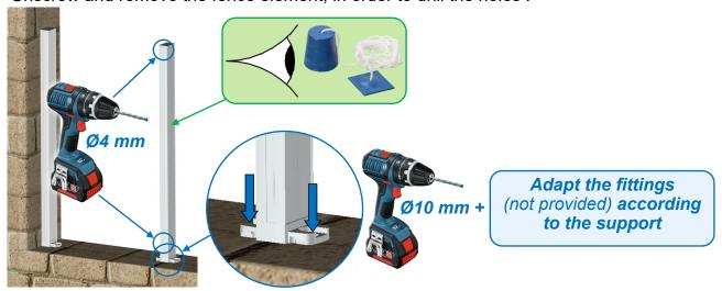
Check the clamp screws on the 2 posts, they must not exceed the bearing plates then attach the screw covers :
