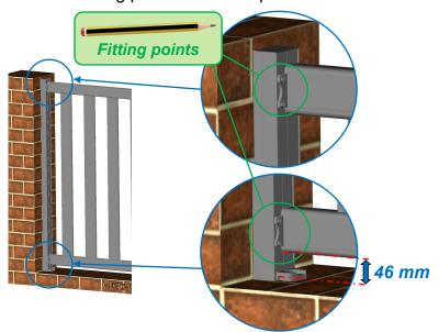
Drill the holes in the 1<sup>st</sup> post and secure the fence element with screws at the top :
