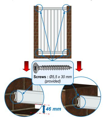
Repeat this process to install the rest of the fence elements.
