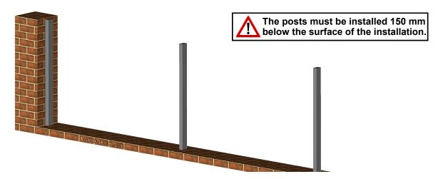
Position the fence element and mark the fitting points :
