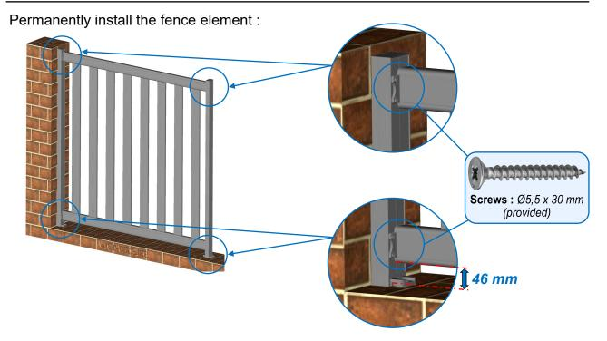
**Resume from chapter :** Drill the 1<sup>st</sup> post, for the installation of the following fence elements.
