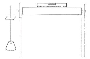
CHECK THAT THE GUIDING RAILS ARE CORRECTLY ALIGNED AND THAT THE AXLE IS PERFECTLY HORIZONTAL
