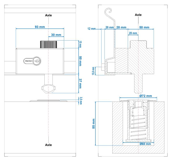
If the end-slat is equipped with a watertight seal or a feeler joint, then it will be impossible to install a floor anchor lock on it.
