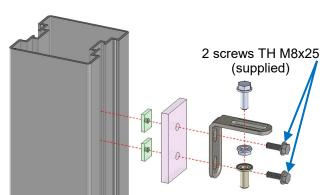
Post 120x120 to seal or screw or 220x220 to seal
