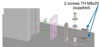
Post 120x120 to seal or screw or 220x220 to seal
