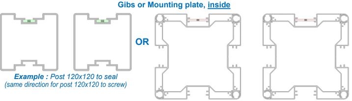
**Example :** Post 220x220 to screw (same direction for post 220x220 to seal)
