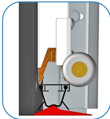
Weather seal section to be glued to the floor between the rails.
