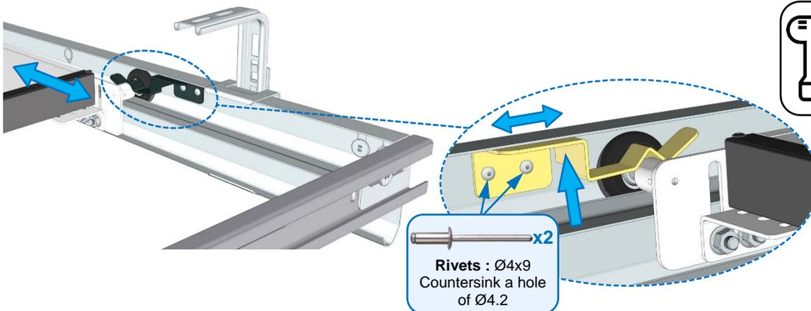
**Rivets : Ø4x9 Countersink a hole of Ø4.2 x2**
