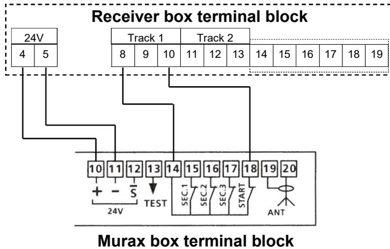
**Connection with an Axovia 220A or B operator**
