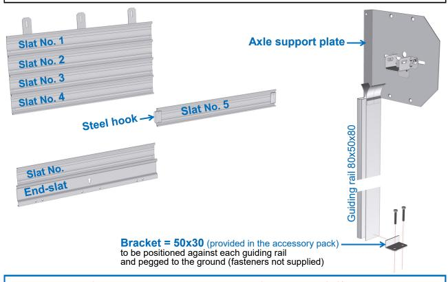
No. of slats with steel hooks, for axle of Ø133 mm 5 - 9 - 13 - 18 - 23 - 28 - 33 - 38 - 43 - 48 - 53 - 58 - 60 - 64 - 69 - 72 - 77
