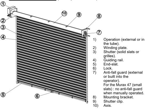
(Shutter diagram Murax hollow axis parachuted with BOX operator)
